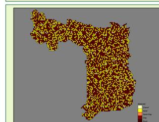
Figure 9 Realization of the aquifer heterogeneity
