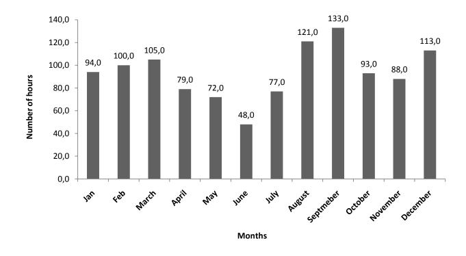
Figure 2 - Average hours of operation of solar pumps across months in 2013
