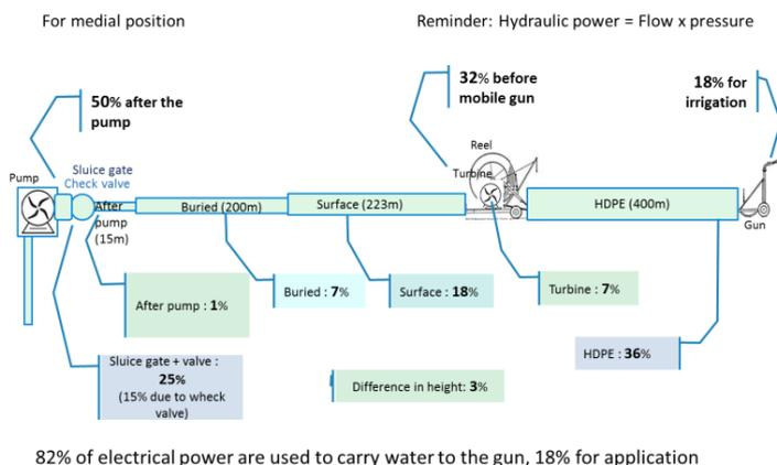
Figure 4: energy loss distribution on the mobile gun installation
