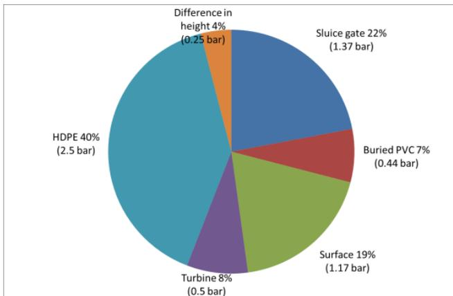
Figure 6: Example of pressure loss in a studied installation
