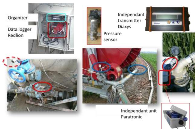
Figure 3: equipment used on measurement chain
