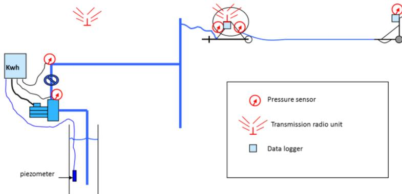
Figure 2: measurement chain on mobile gun
