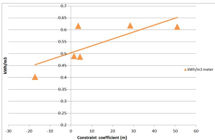
Figure 7: Relation between kWh/m<sup>3</sup> “meter” and constraint coefficient
