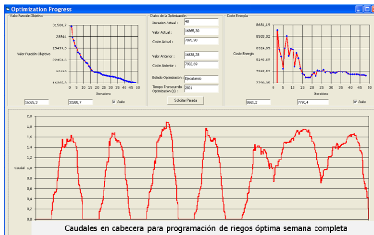
Figure 4. Timeline of flow rates in the pumping station for a schedule optimised for a full week, showing the hydraulic and energy convergence indicators
