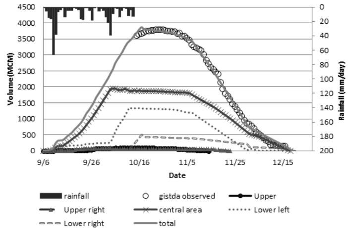
Fig. 6 Estimation of flood volume in the target paddy areas during the flood in 2011
