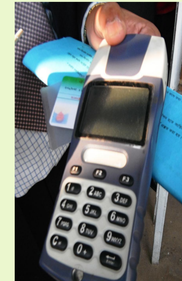
Recharging a farmer's smart card for pre-paid meter
