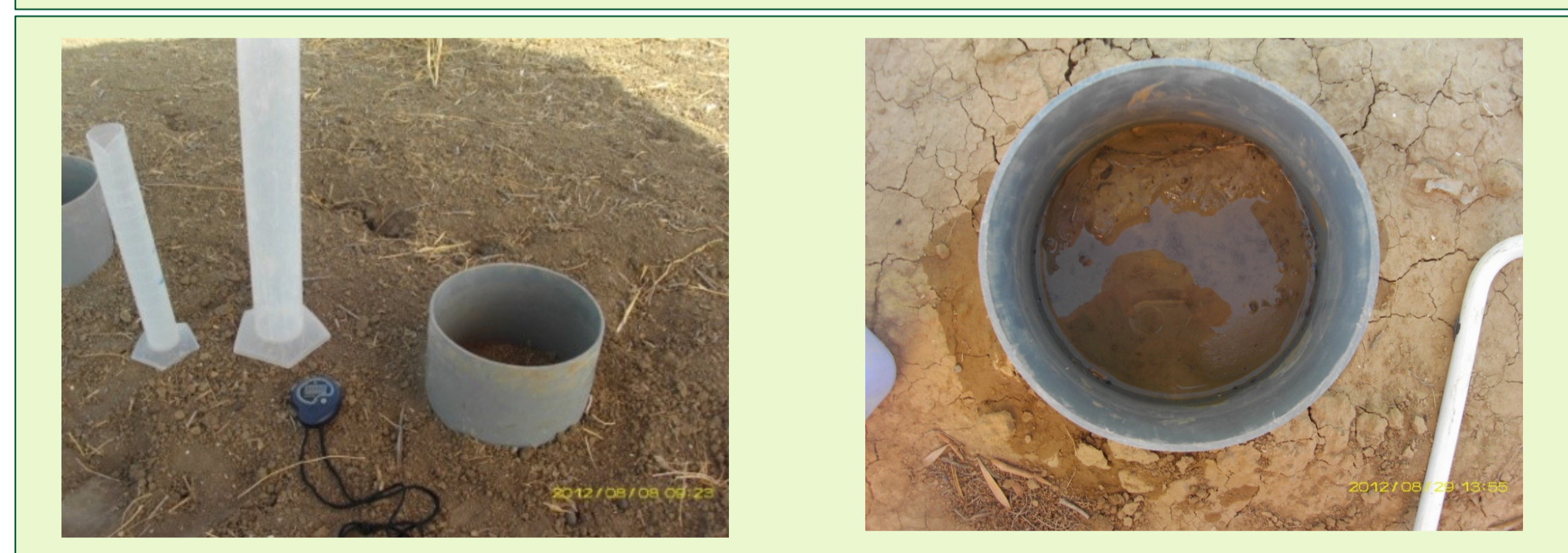
Infiltration tests with the Beerkan method
