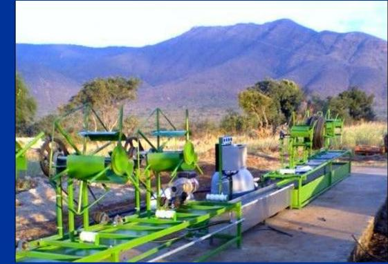
What the ultrasonic sound does is create millions of tiny vacuum bubbles on every micro surface of the dripline that will then implode in the pipe and cause shockwaves that completely strip all impurities in seconds.
