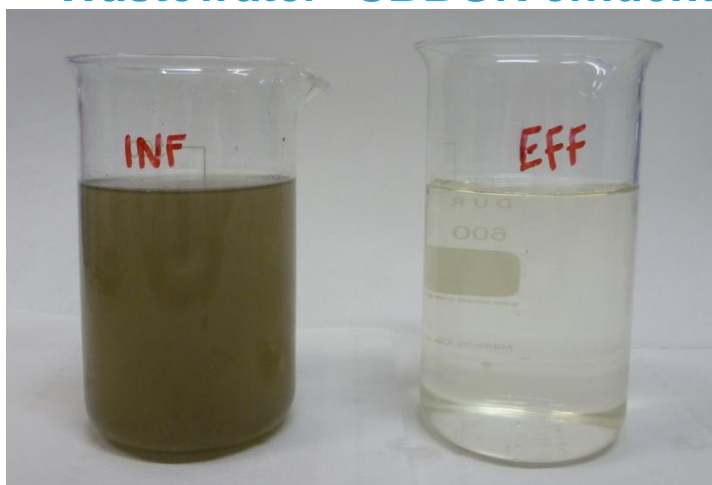
Wastewater SBBGR effluent
