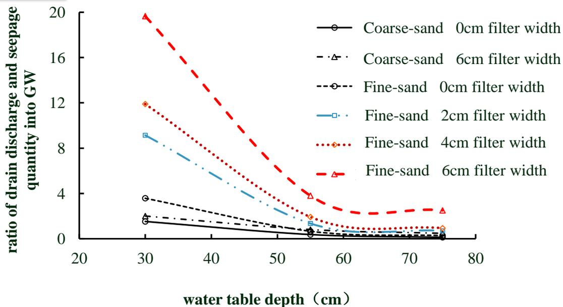
Fig 7. Effects of water table depth on the ratio of drainage and seepage quantity
