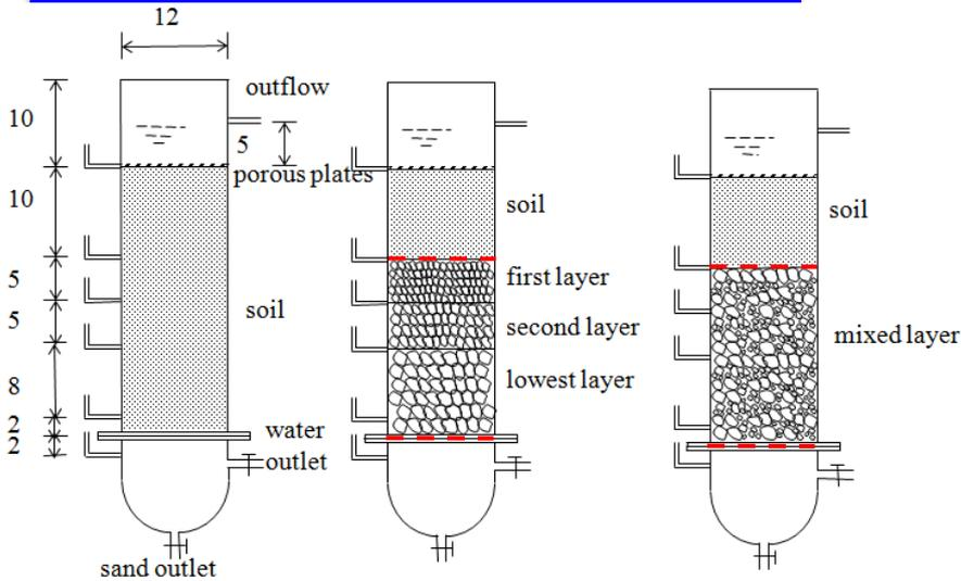
Fig 3. Clogging defense test equipment
