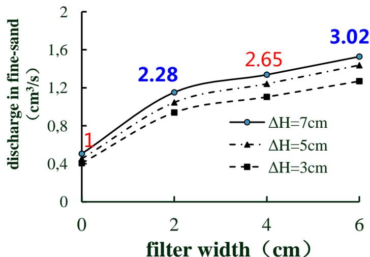
Fig 4. Variation of drain discharge with filter width under different ponding depths
