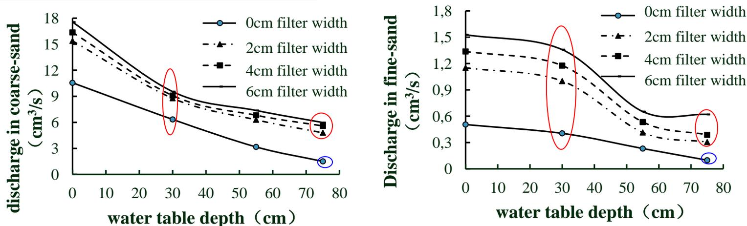
○ Having drainage function still    ○ Almost lost drainage function
