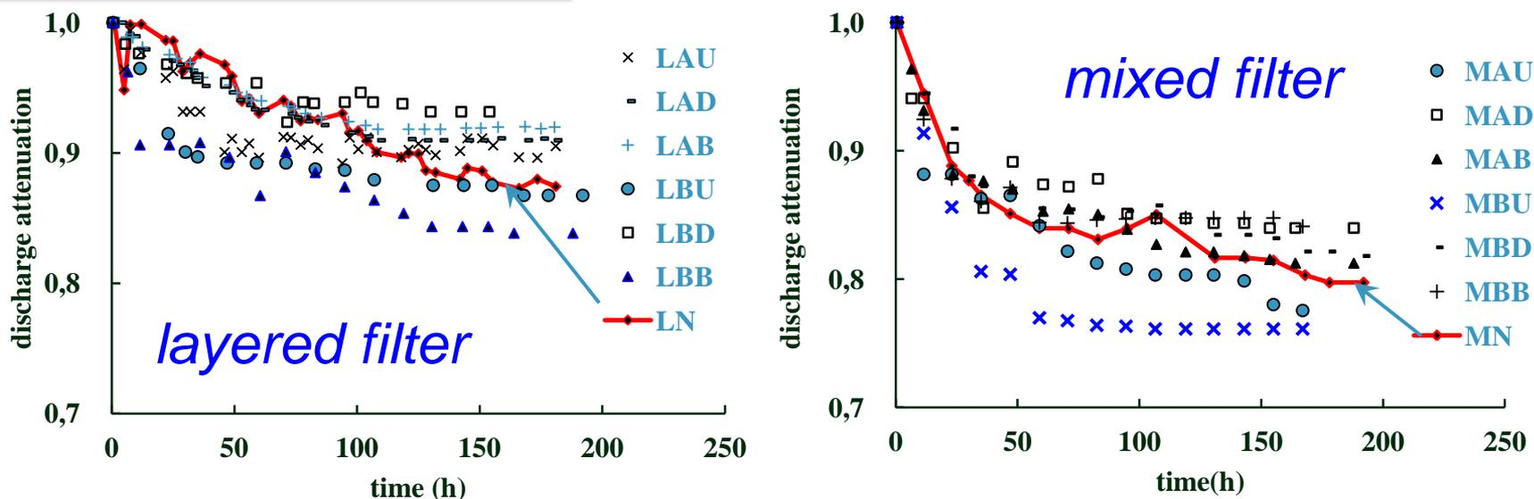
Fig 9. Discharge attenuation under multiple clogging defense measures
