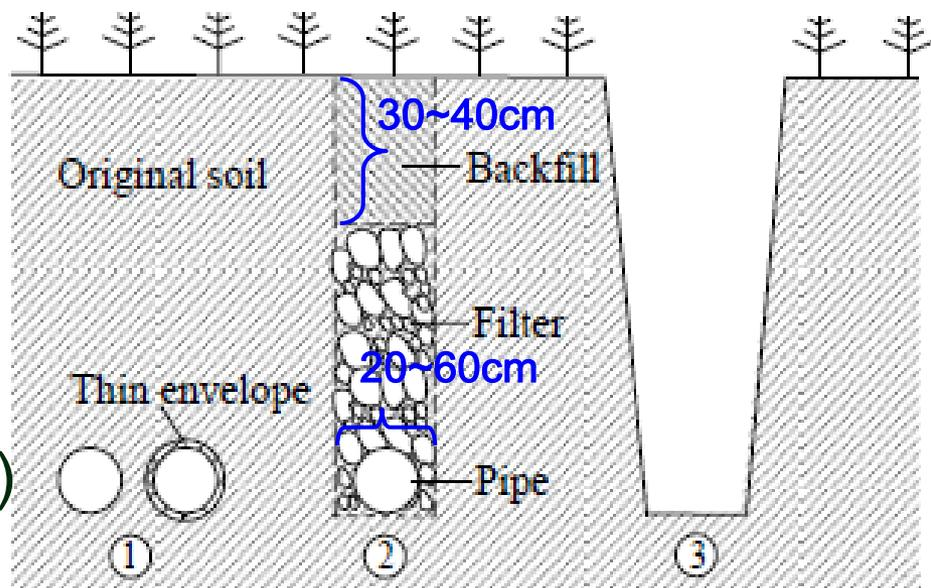
1. Conventional subsurface pipe drainage
