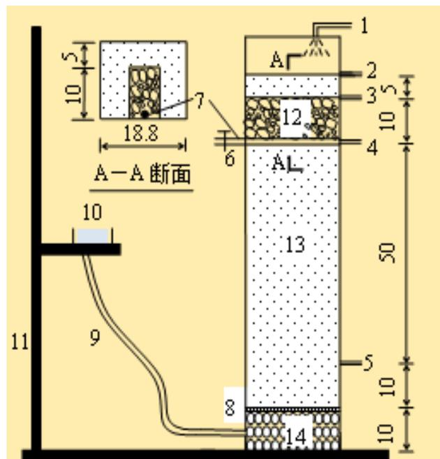
1.Inlet; 2-5. Piezometers; 6.Sealing; 7.Drain pipe; 8.Support network; 9.Connecting tube; 10.Water tank; 11.Removable support; 12.Filter; 13.Soil medium; 14. High permeability material (cm)
